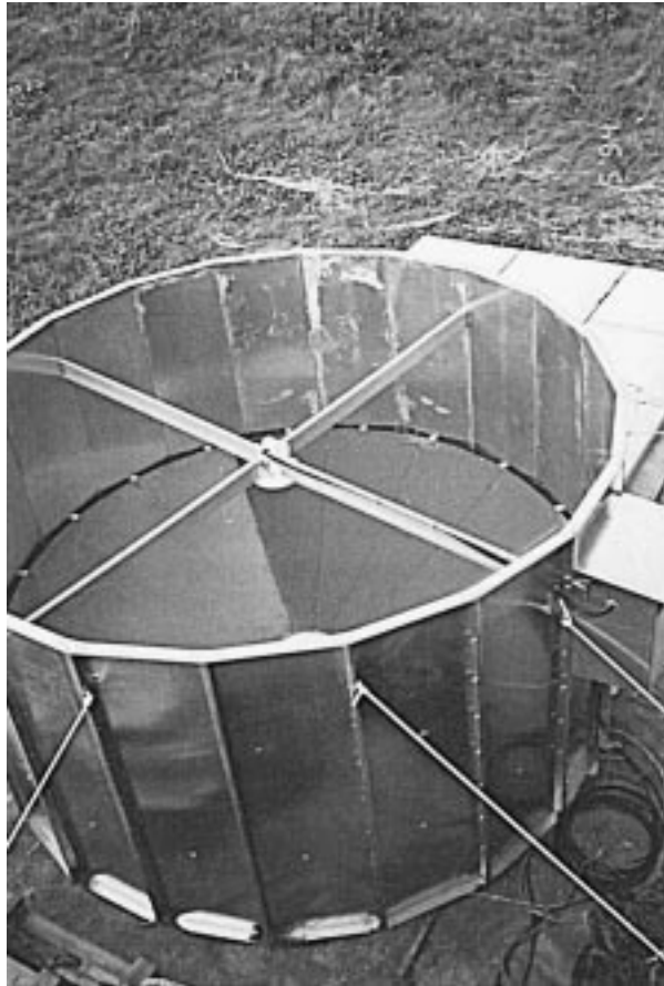
FIG. 1. The 3-GHz profiler dish antenna and shroud as configured for FAO and MCTEX.
