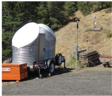
A new vertically pointing snowlevel radar and optical disdrometer have been installed at the Hydrometeorology Testbed (HMT) Los Gatos soil moisture site to help improve precipitation estimation with the Santa Clara AQPI X-band precipitation scanning radar.
